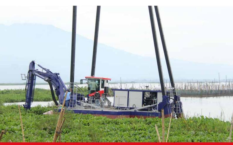
Italdraghe, based on the pluriannual experience of cutter suction dredger production, has developed the multifunctional amphibious dredger in order to perform all shallow water work from dry ground to water and marshy/muddy soils. This dredger is specifically designed for multi purposes work with only one machine – water work, for working from the land side, suction dredging, excavating, raking and pile-driving.
