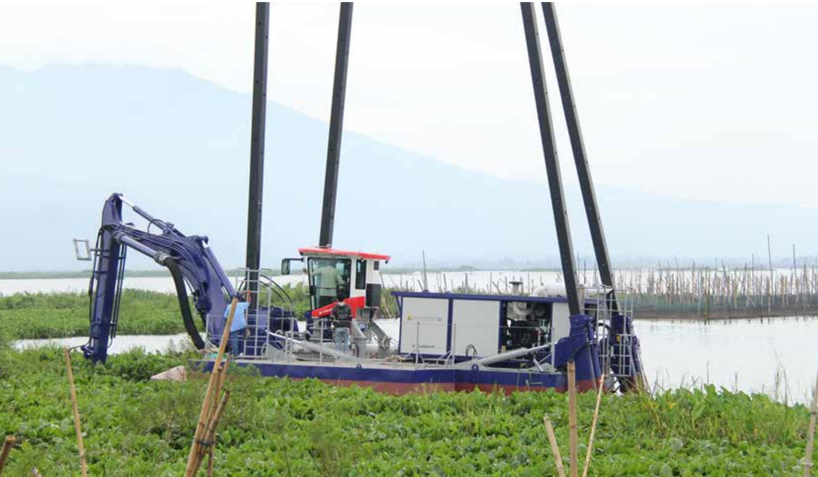
Italdraghe, based on the pluriannual experience of cutter suction dredger production, has developed the multifunctional amphibious dredger in order to perform all shallow water work from dry ground to water and marshy/muddy soils. This dredger is specifically designed for multi purposes work with only one machine – water work, for working from the land side, suction dredging, excavating, raking and pile-driving.
