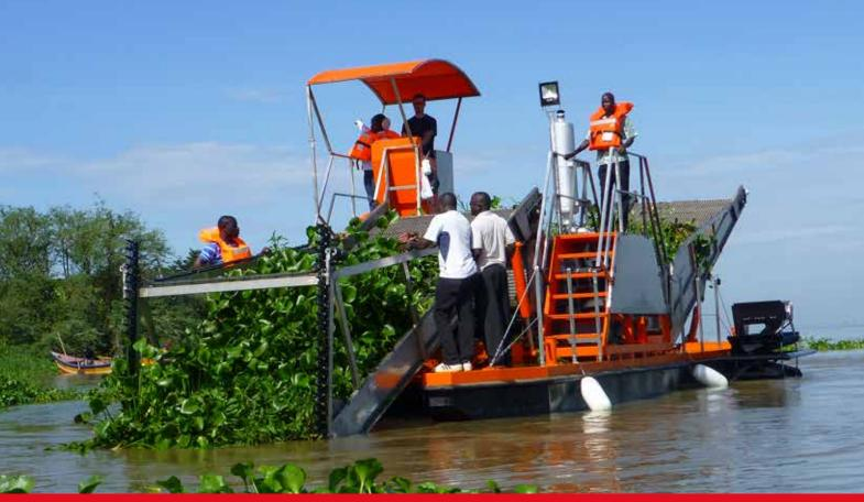
Kenya harvester is a machine designed for harvesting materials such as weeds and hyacinths that obstruct the passage of water in lakes, rivers and canals. Additionally, the harvester can be used as a skimmer for the harvesting of floating rubbish such as plastic and glass bottles, pieces of wood, cans and other materials.
