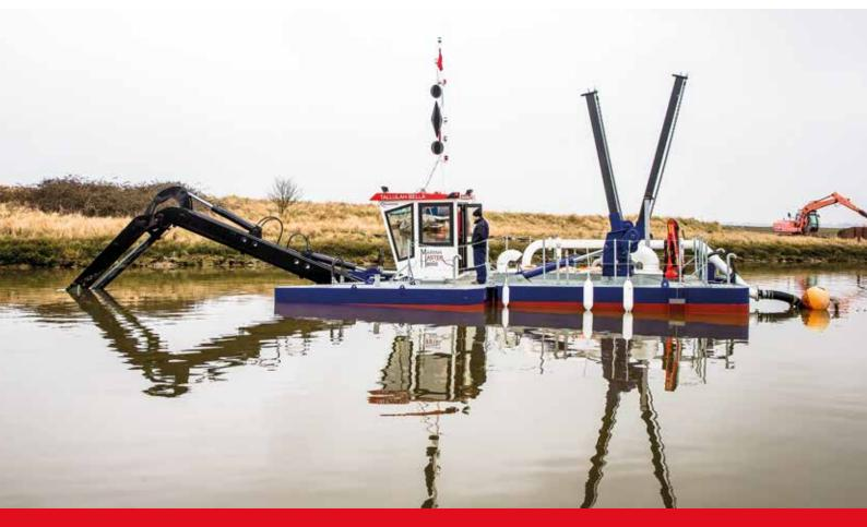
Italdraghe has developed and designed the marina master dredger in order to allow to operate under floating docks and floating piers where a different type of dredger would not be able to operate due to limited manoeuvrability chances.
