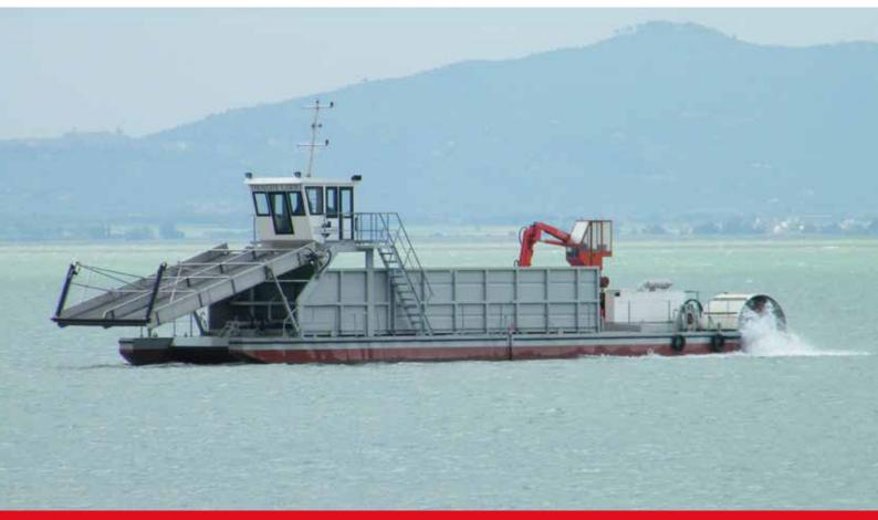
Trasimeno harvester is a machine designed for harvesting materials such as weeds and hyacinths that obstruct the passage of water in lakes, rivers and canals. Additionally, the harvester can be used as a skimmer for the harvesting of floating rubbish such as plastic and glass bottles, pieces of wood, cans and other materials.
