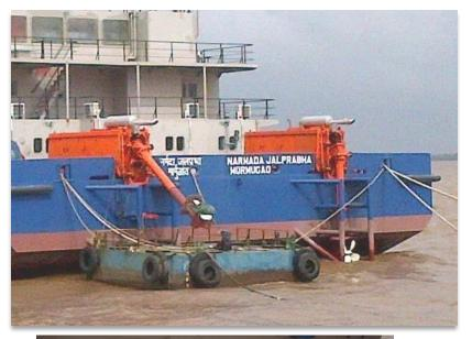
ITALDRAGHE SpA's mechanical and hydraulic azimuthal rudder propellers offer the benefits of a combined propulsion and steering system.
