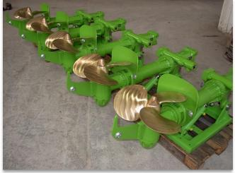
They are fitted with immersion adjustment and trim systems, for routine inspections and maintenance.
