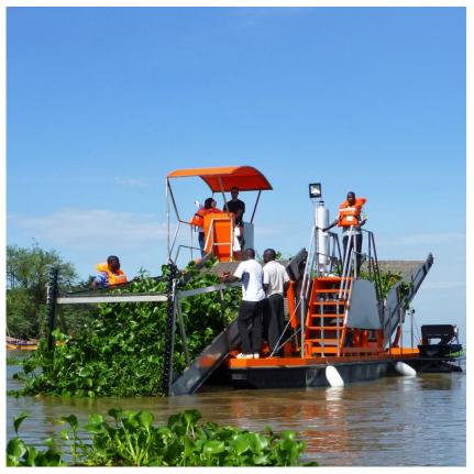
ITALDRAGHE SpA's has a long history of designing and building special purpose work boats, including weed harvesters and garbage collectors for removing rubbish and other floating materials from ports, lakes and canals.
