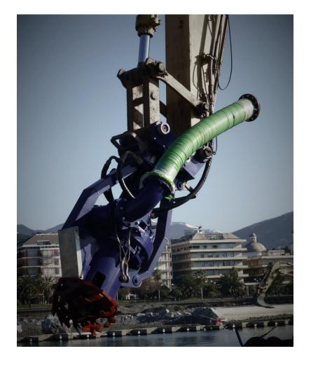
Dredging heads (BD) are basically dredgers in miniature: easy to use, with low maintenance costs and compatible with all brands of hydraulic excavators, this product is ideal for small-scale dredging projects.
